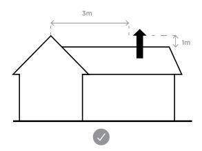
➤ The minimum height of the flue system further than 3 meters from the highest point of the roof shall be 1 meter above roof penetration.
